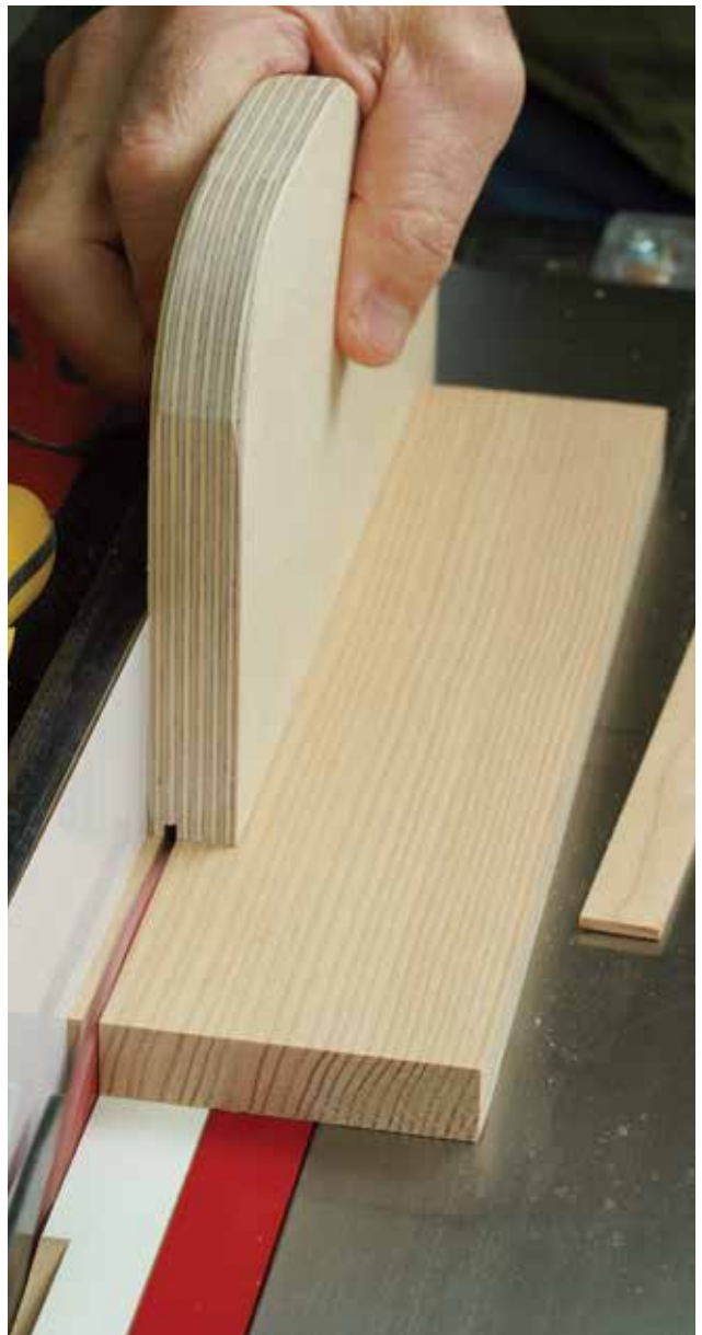
Make thin rips with no worries. With zero clearance around the blade, the thinnest ripcuts can be made safely and cleanly. Note how a fresh push stick carries both parts past the blade.
