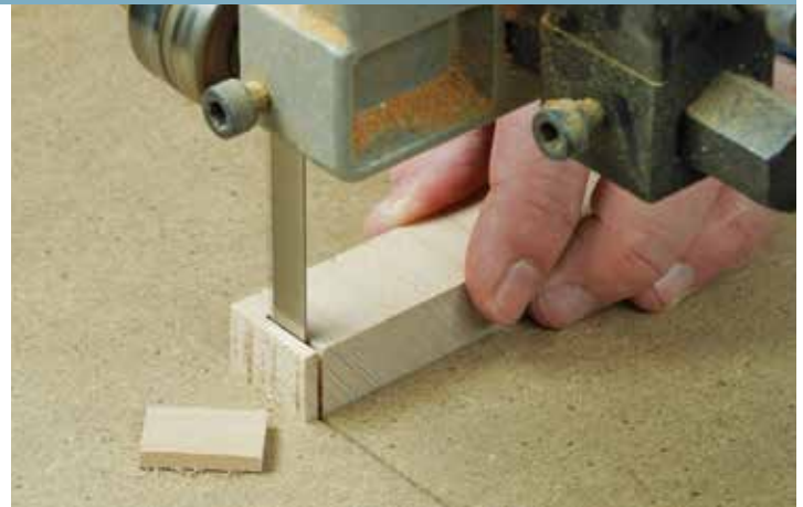
Zero clearance at the bandsaw. Cut partway into a piece of \frac{1}{4} -in. MDF, then clamp it in place to create support around the blade.
