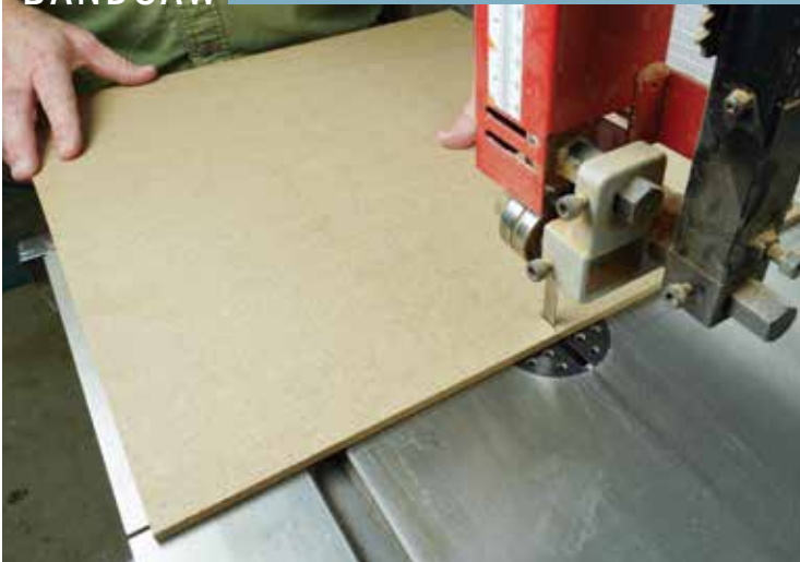
Zero clearance at the bandsaw. Cut partway into a piece of \frac{1}{4} -in. MDF, then clamp it in place to create support around the blade.
