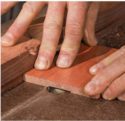
Spandrel gets a sliding dovetail. On the inside face of the spandrel, Cameron routs a shallow sliding dovetail socket. The leg will lock into it.
