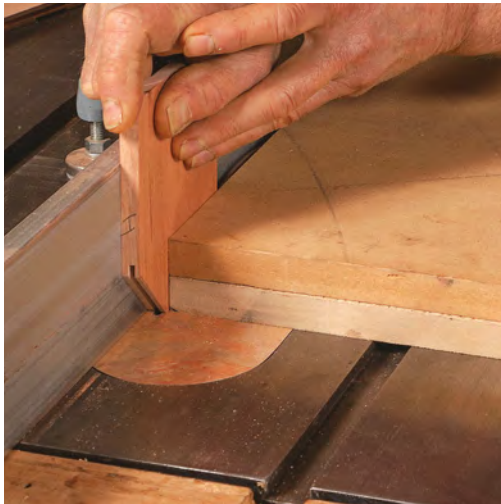
The slot in the spandrel. The top of the spandrel gets slotted, allowing it to slide onto the apron in a bridge joint. Cameron makes the cut at the table saw, clamping sheet goods to the saw as a second fence.
