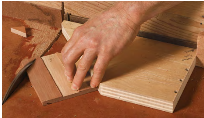
Mismatched miters. Because the legs are splayed at 1.5^\circ , the two miters on the spandrel differ. Cameron lays them out with knife lines, cutting one at 44.25^\circ , the other at 45.75^\circ . When the miters are done, he'll crosscut the top of the spandrel 1.5^\circ off 90^\circ .
