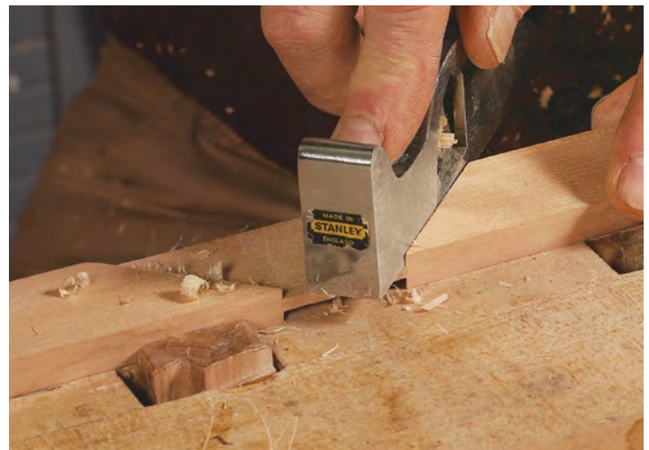
Double bevel transfer. Cameron uses a pair of bevel gauges to transfer the miter angles from the spandrel to the apron (top). After removing most of the waste with a handheld router, cutting close to his layout lines, Cameron finishes the apron half of the mitered bridge joint with chisels and shoulder planes (above).
