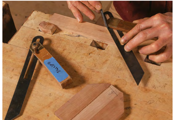
Mismatched miters. Because the legs are splayed at 1.5^\circ , the two miters on the spandrel differ. Cameron lays them out with knife lines, cutting one at 44.25^\circ , the other at 45.75^\circ . When the miters are done, he'll crosscut the top of the spandrel 1.5^\circ off 90^\circ .
