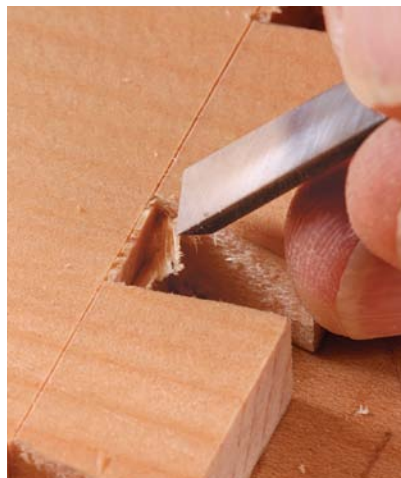
Hand power. When paring by hand, place the chisel with your forward hand and drive it with your rear hand. Keep your body weight behind the tool to help (left). It is especially important to take thin cuts so the chisel won't bog down in the cut (above).
