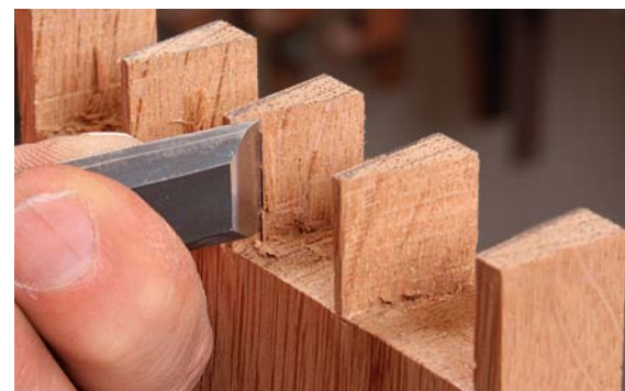
Pare down if the grain allows it. When cleaning up pins, it's easiest to pare straight down (top). To prevent tearout when the grain is angled in, pare side-to-side across the grain (bottom).
