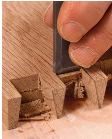
Thin slices, even when chopping. Work back to the baseline, taking \frac{1}{32} -in. cuts. Angle the chisel to undercut the joint slightly to ensure the joint seats fully. Work halfway, then flip the stock and finish up from the other side.
