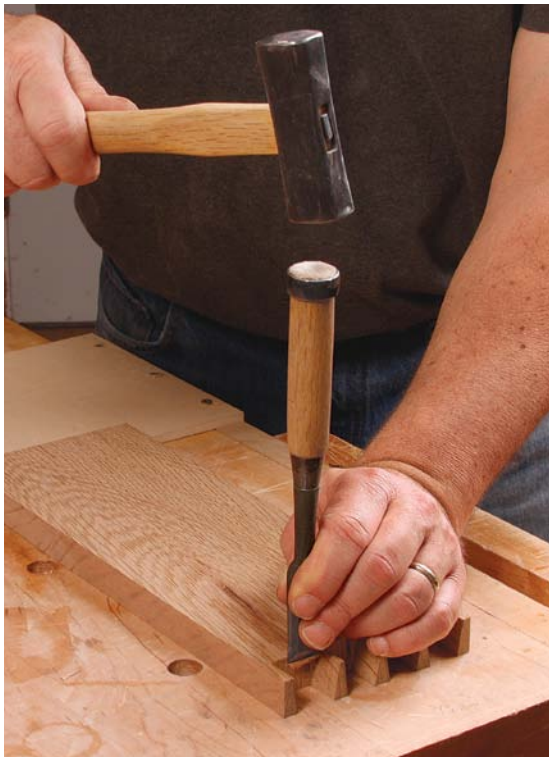
Grip it low for control. Pinch the blade near the tip and rest your hand against the stock when placing the chisel.
