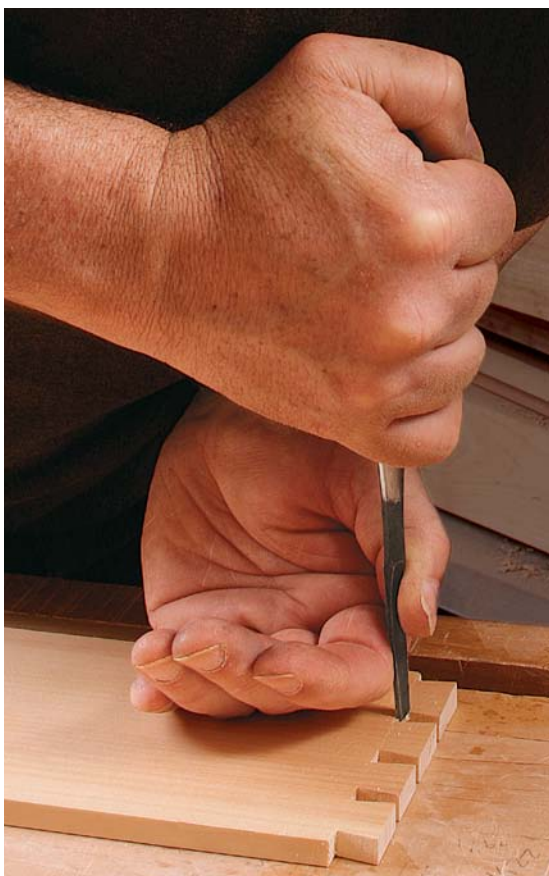
Grip it low for control. Pinch the blade near the tip and rest your hand against the stock when placing the chisel.
