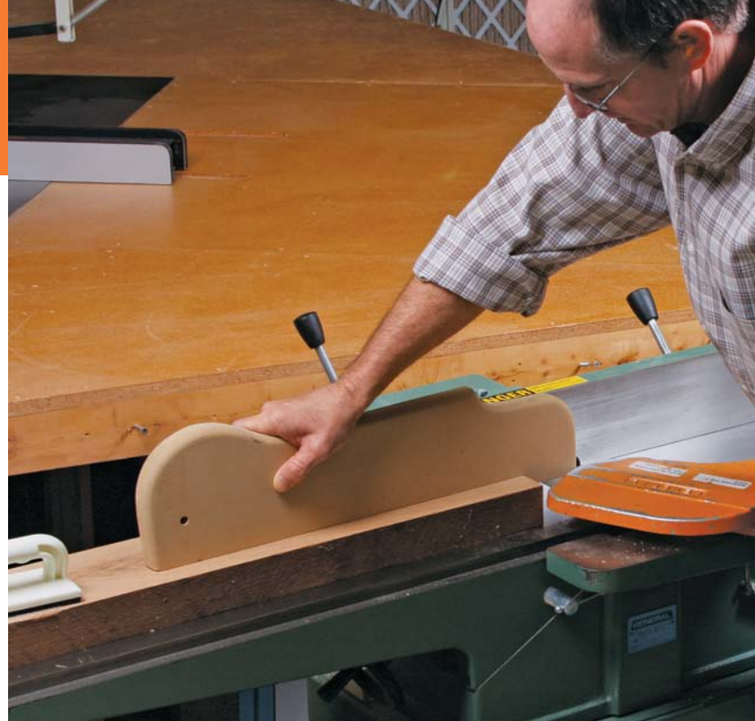
4 Finish the cut. A long push stick will maintain a good grip and good downward pressure as you finish the pass.
