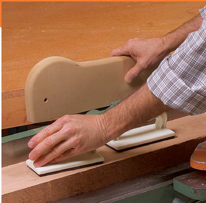
3 Grab the push stick. When the end of the board draws closer, reach for the push stick while keeping the stock moving.
