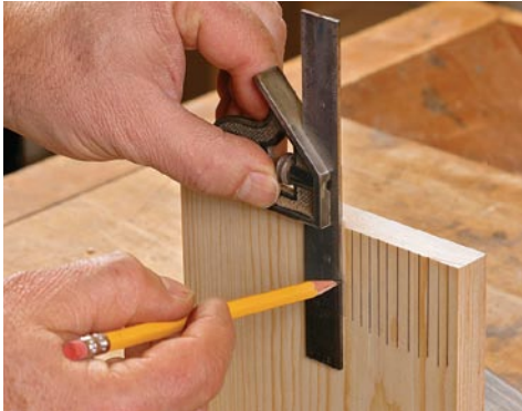
For square cuts, start with a square setup. Clamp a board in the vise using a square for alignment. Then use the square to draw lines on the board's face. With plumb lines as a guide, you're ready to start sawing.
